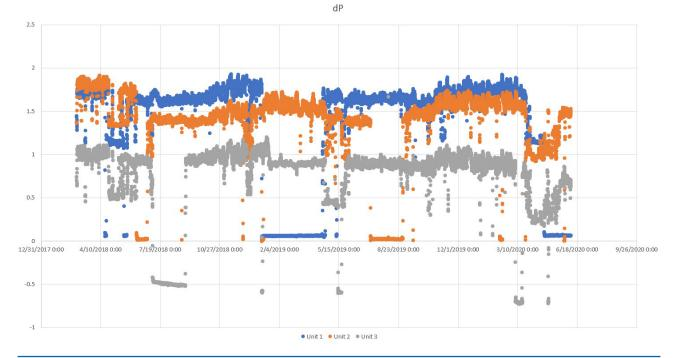
Figure 3. This graph demonstrates that three units with the same exact design, operating at the same time, can have different running parameters based on SCR performance.
