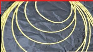
**1** The PRIMACORD detonating cord curtain application is tailored to each unit based on area size, plus the amount and nature of the fouling.
